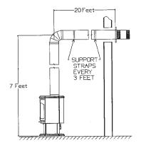
The maximum horizontal vent run with one 90° elbow attached is 20 feet with 8 feet vertical.
