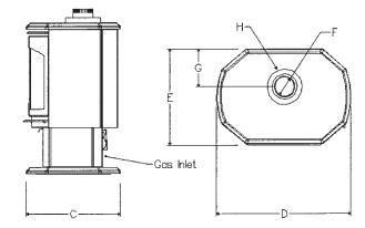
Gas inlet is located on the back of the unit.
