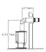
The minimum allowable configuration is  $4^{1}/2$  feet vertical with unit 4" from wall.
