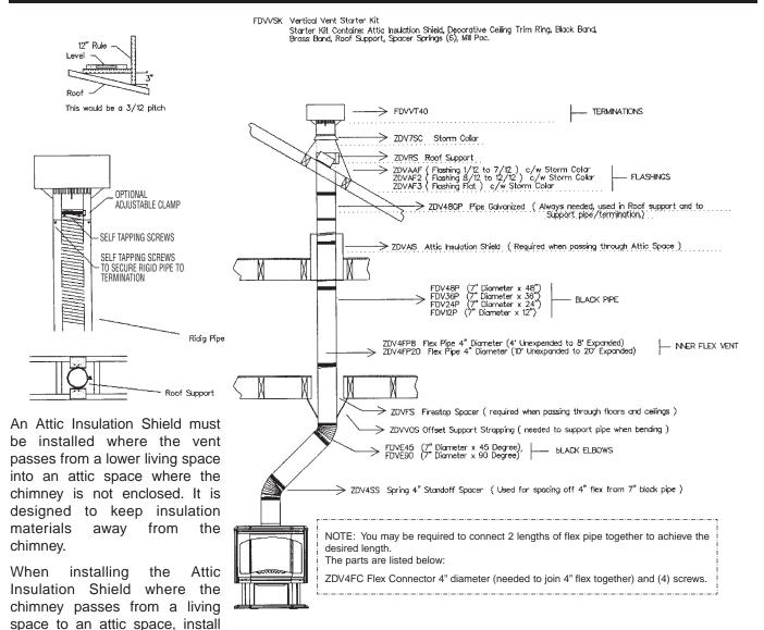
the shield from below and nail it in place using 1" spiral nails.
