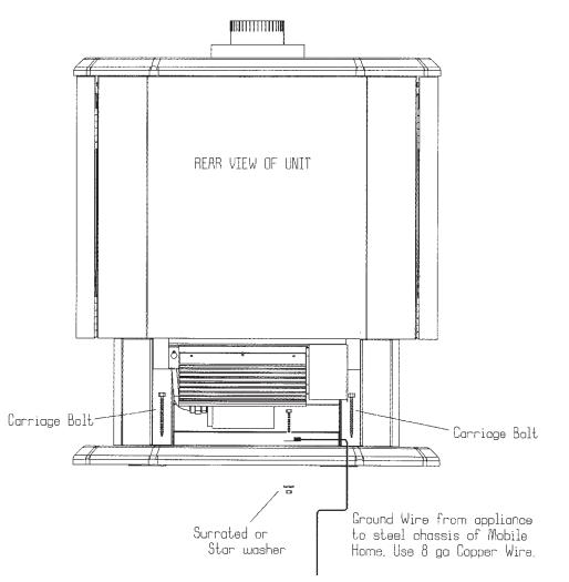
THE FDV350N AND FDV350LP MAY BE INSTALLED IN MANUFACTURED (MOBILE) HOMES AFTER FIRST SALE. THE MODELS CONVERTED USING THE B-VENT CONVERTER CANNOT BE INSTALLED IN A MANUFACTURED (MOBILE) HOME.
